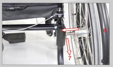
Assemble the rear wheel with push rims (6) on the side that suits the user. Enter the rear wheel axle into the attachment and at the same time pulling out the locking pin (7). Check that the axle is fully inserted. Repeat on the other wheel.
