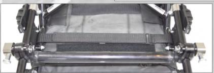
Disassemble the rear wheels and put the wheelchair up side down to access the rear axle. One arm drive with QR is mounted together with the steel rear axle, and if the chair is equipped with the Carbon rear axle, you need to replace it with the steel rear axle.
