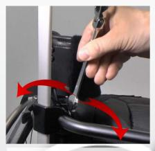
6) Use a 10 mm spanner and turn the metal cup forwards or backwrads until the oush handle is vertical.
