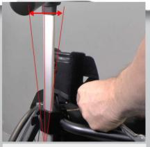
5) If the angle of the push handle needs to be adjusted, you can turn the excentric metal cup with a 10 mm spanner.. Start with loosen the screw that holds the attachment, a bit.
