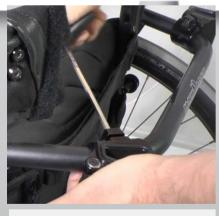
4) Tighten the screw with allen key 4 mm. Repeat the procedure on the right side.
