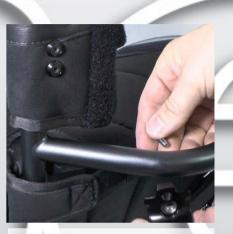
3) Open up the attachment and place it around the backrest tube, and let the metal cup guide the attachment onto the knob at the backside of the tube. Fold the attachment and mount the M5 screw.
