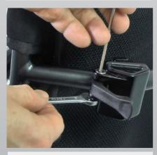
4) Adjust the locking force by turning the nut anti-clockwise (seen from the top) to encrease it, and clockwise to decrease the locking force. Turn the nut a quarter of a turn, using a 8 mm spanner, tighten the screw and test it.
