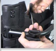
5) Then mount the larger M5 screw in the upper hole, that holds the attachment together, with allen key 4 mm. Then tighten both the M4 and M5 screws firmly. Repeat the procedure on the other side.
