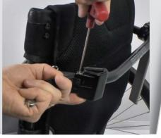
2) Disassemble the push handle. Loose this screw a few turns with allen key 2.5 mm.
