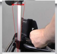
5) If the angle of the push handle needs to be adjusted, you can turn the excentric metal cup with a 10 mm spanner.. Start with loosen the screw that holds the attachment, a bit.
