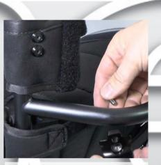
3) Open the attachment and place it around the backrest tube. Let the metal cup guide the attachment onto the knob on the backside och the tube. Mount the smaller M4 screw through the metal cup into the threaded knob
