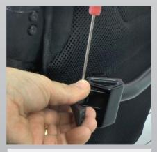
5) Tighten the screw and make sure that the nut slides into the attachmnet properly.
