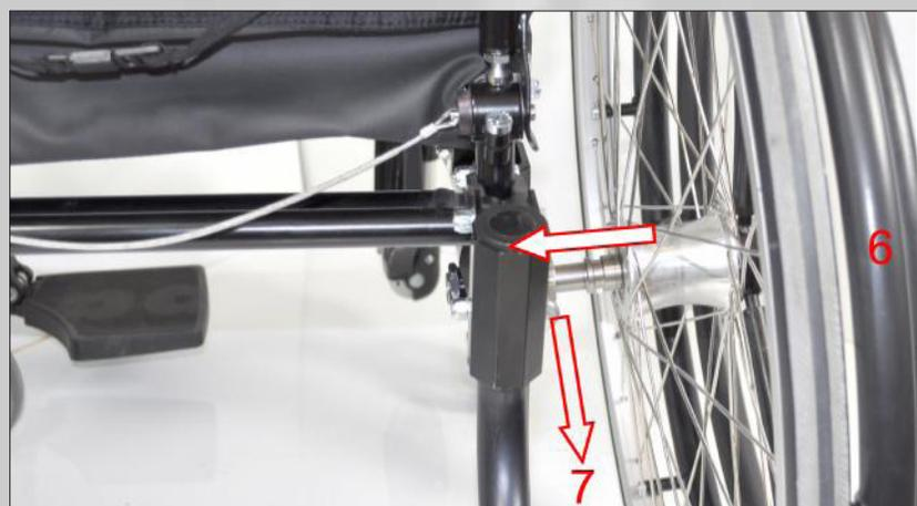
Assemble the rear wheel with push rims (6) on the side that suits the user. Enter the rear wheel axle into the attachment and at the same time pulling out the locking pin (7). Check that the axle is fully inserted. Repeat on the other wheel.
