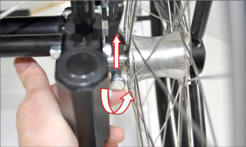
Turn the locking pin and check that it enters fully and lock the rear wheel. Check on both sides. **NOTE! Important!**
