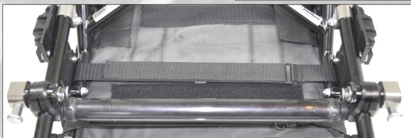
Disassemble the rear wheels and put the wheelchair up side down to access the rear axle. One arm drive with QR is mounted together with the old std rear axle, and if the chair is equipped with the Carbon rear axle, you need to replace it with the old std rear axle.
