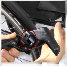
1) The attachment for the brake should be mounted around the chassis tube.
