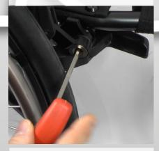
6) When the brake is properly adjusted tighten the screw firmly with allen key 5
