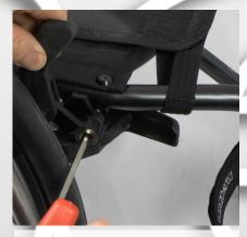
3) Tighten the screw slightly with allen key 5 mm.
