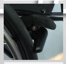
4) Engange the brake and check that the brake blade cuts into the pumped tire approx. 5 mm.
