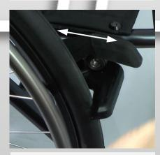
5) If needed adjust the brake in depth to get the correct brake force.
