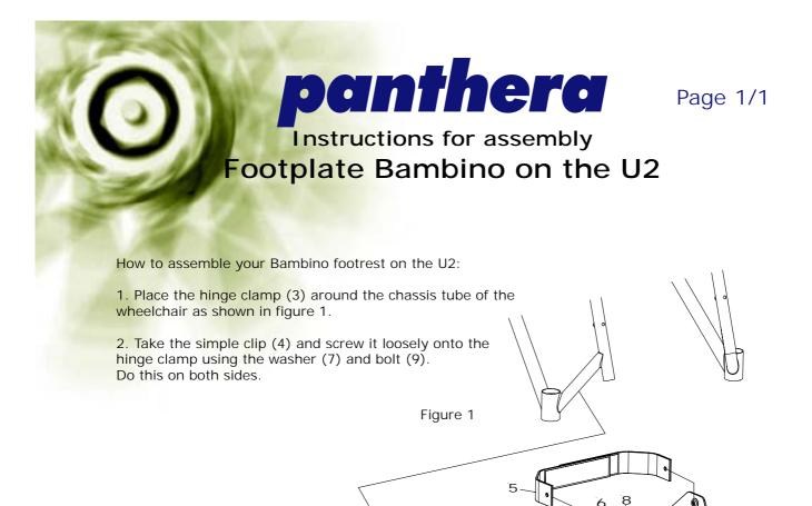
3. Then position "the Bambino footrest mounting" (2) in the "simple clip" (4). Do this on both sides.
