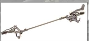
The new X brake is designed to be mounted on Panthera X in the brackets, seen in **image 1**. The brackets are located on the underside of the frame tubes at the front, on both sides of the chassis.
