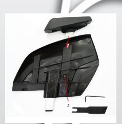
2) 2) The armrest is put into the hole where the end plug was located. Put the nut for adjusting the armrest (pos 4) in its groove in front side. Refit the spring (pos 3, fig 1) and the screw (pos 2) on the back. Only screw in the screw a few turns.
