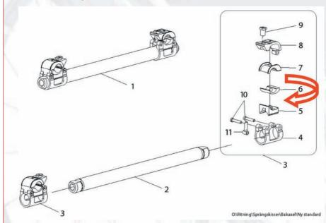
The std length of the Carbob axle (+15mm) should be mounted with the plastic parts 6 and 7 as the image shows.
