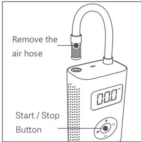
3. Connecting the High-pressure Air Hose and Nozzle
