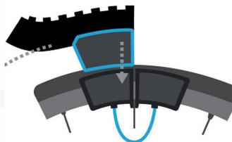
Attach one end of reTyre Traction skin to one half of the mounting clip and roll on to reTyre Traction. Make sure the reTyre Traction embraces the Tyre.
