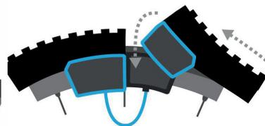
After the full turn of the wheel, pull the end and attach the velcro ends to the other half of the mounting clip. Now the reTyre Traction is mounted and there should be a gap of 0-20mm in the seam.
