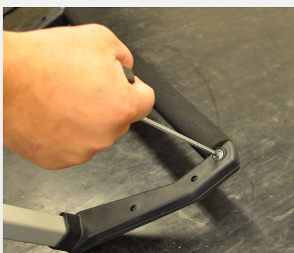
Fig. 18 Loosen the screw on one side with allenkey 4 mm.
