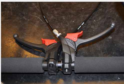
Fig. 23 If the brake handle is short, 33 cm or below, you might need to mount the handles as shown in the image to make room.
