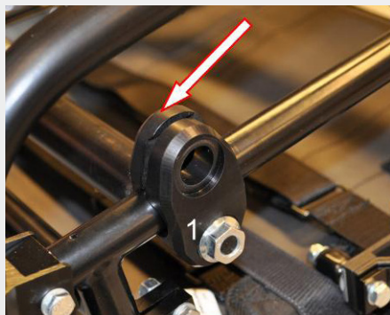
Fig. 1 Mount the old std rear axle , (if not already done) and switch the inner wheel bracket, on both sides, with brackets included (art.no. 3300010). Tighten the nut (1) slightly.
