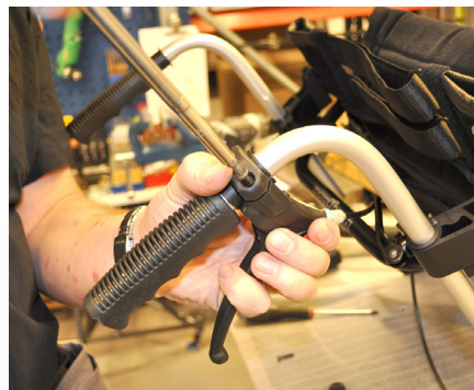
Fig. 14 Mount the brake handles on the push handles.
