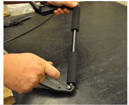
Fig. 22 Remount the two foam parts on the push-handle.
