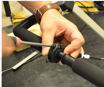
Fig. 21 Mount the brake handles and tighten the screws.
