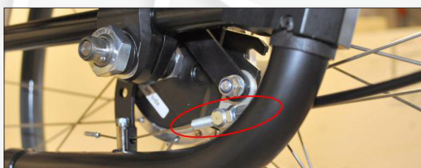
Fig. 15 Adjust the brakes with the screws by the brake handles and by the brake linings. Justera bromsarna med skruvarna vid bromshandtaget resp. bromsbackarna.
