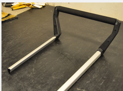
Fig. 17 Remove the push bar from the wheelchair
