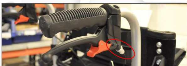
Fig. 13 Mount the push handles on the brackets at the back rest and pull the wires through the back rest upholstery.
