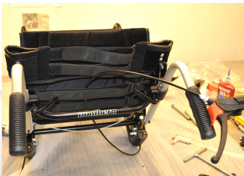
Fig. 13 Mount the push handles on the brackets at the back rest and pull the wires through the back rest upholstery.
