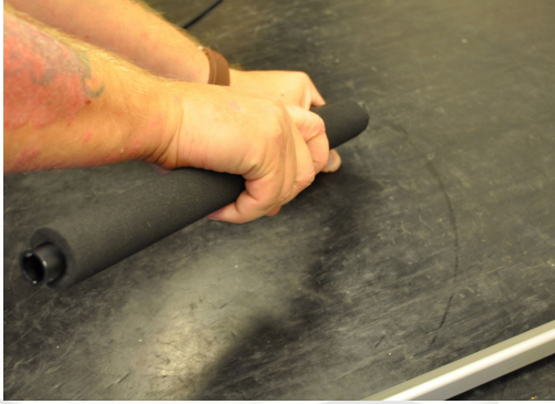
Fig. 20 Pull off the foam from the pushbar.
