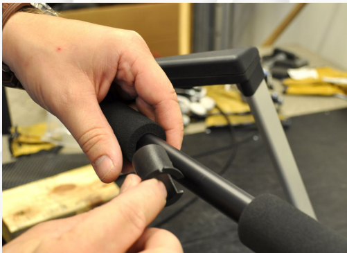
Fig. 20 Mount the plastic sockets that comes with brake kit, on both sides of the push handle.
