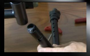
Enter the anti-tip into the chassis.
