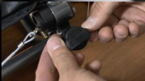
Finally mount the knob and tighten the screw with allen key 3 mm.
