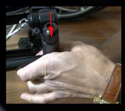
Pull out the anti-tip from the chassis.
