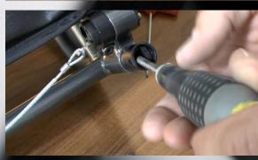
Then use a screwdriver and turn the tube 1/4 of a turn anti clockwise (on the right side, clockwise on the left), until the tube enter a slot and slide down an additional distance.
