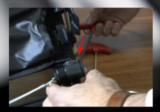
Remove the screw that holds the anti-tip to the chassis with allen key 5 mm.
