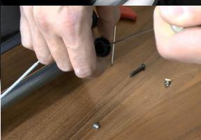
Use a spoke from a rearwheel and hold the tube while removing the rivet or screw, and then let the tube slide into the chassis.
